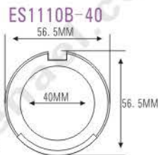
ES1110B-40 ES1110B-36 SIZE: \varnothing 56.5 \times H12.3\text{mm}
